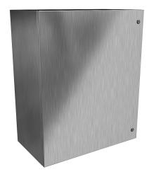
Hammond Eclipse series enclosure, NEMA 3R/4/4X/12/13, 36 x 30 x 16in (HxWxD), wall mount, 304 stainless steel, #4 brush finish, single-door, 1/4-turn semi-flush 316 stainless steel latch.
