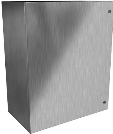
Hammond Eclipse series enclosure, NEMA 3R/4/4X/12/13, 36 x 30 x 16in (HxWxD), wall mount, 304 stainless steel, #4 brush finish, single-door, 1/4-turn semi-flush 316 stainless steel latch.
