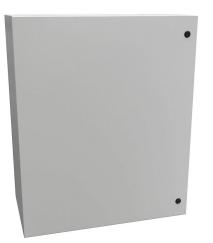
Hammond Eclipse series enclosure, NEMA 3R/4/12, 36 x 30 x 16in (HxWxD), wall mount, carbon steel, RAL 7035 light gray, powder coat finish, single-door, 1/4-turn semi-flush latch.
