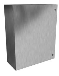
Hammond Eclipse series enclosure, NEMA 3R/4/4X/12/13,  $36 \times 30 \times 12$ in (HxWxD), wall mount, 316 stainless steel, #4 brush finish, single-door, 1/4-turn semi-flush 316 stainless steel latch.
