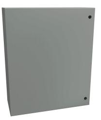
Hammond Eclipse series enclosure, NEMA 3R/4/12, 36 x 30 x 12in (HxWxD), wall mount, carbon steel, ANSI 61 gray, powder coat finish, single-door, 1/4-turn semi-flush latch.
