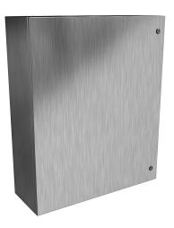
Hammond Eclipse series enclosure, NEMA 3R/4/4X/12/13,  $36 \times 30 \times 10$  in (HxWxD), wall mount, 316 stainless steel, #4 brush finish, single-door, 1/4-turn semi-flush 316 stainless steel latch.
