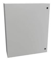
Hammond Eclipse series enclosure, NEMA 3R/4/12,  $36 \times 30 \times 10$ in (HxWxD), wall mount, carbon steel, RAL 7035 light gray, powder coat finish, single-door, 1/4-turn semi-flush latch.
