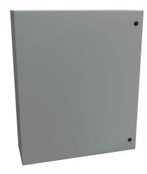
Hammond Eclipse series enclosure, NEMA 3R/4/12,  $36 \times 30 \times 10$ in (HxWxD), wall mount, carbon steel, ANSI 61 gray, powder coat finish, single-door, 1/4-turn semi-flush latch.
