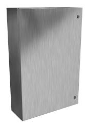
Hammond Eclipse series enclosure, NEMA 3R/4/4X/12/13, 36 x 24 x 8in (HxWxD), wall mount, 316 stainless steel, #4 brush finish, single-door, 1/4-turn semi-flush 316 stainless steel latch.
