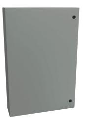
Hammond Eclipse series enclosure, NEMA 3R/4/12,  $36 \times 24 \times 6in$  (HxWxD), wall mount, carbon steel, ANSI 61 gray, powder coat finish, single-door, 1/4-turn semi-flush latch.
