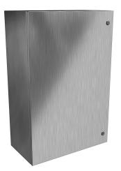
Hammond Eclipse series enclosure, NEMA 3R/4/4X/12/13,  $36 \times 24 \times 12$ in (HxWxD), wall mount, 304 stainless steel, #4 brush finish, single-door, 1/4-turn semi-flush 316 stainless steel latch.
