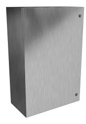
Hammond Eclipse series enclosure, NEMA 3R/4/4X/12/13,  $36 \times 24 \times 12$ in (HxWxD), wall mount, 316 stainless steel, #4 brush finish, single-door, 1/4-turn semi-flush 316 stainless steel latch.
