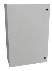
Hammond Eclipse series enclosure, NEMA 3R/4/12,  $36 \times 24 \times 12$ in (HxWxD), wall mount, carbon steel, RAL 7035 light gray, powder coat finish, single-door, 1/4-turn semi-flush latch.
