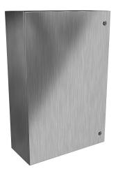
Hammond Eclipse series enclosure, NEMA 3R/4/4X/12/13,  $36 \times 24 \times 10$  in (HxWxD), wall mount, 304 stainless steel, #4 brush finish, single-door, 1/4-turn semi-flush 316 stainless steel latch.
