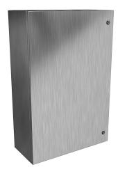
Hammond Eclipse series enclosure, NEMA 3R/4/4X/12/13,  $36 \times 24 \times 10$  in (HxWxD), wall mount, 316 stainless steel, #4 brush finish, single-door, 1/4-turn semi-flush 316 stainless steel latch.
