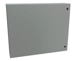
Hammond Eclipse series enclosure, NEMA 3R/4/12,  $30 \times 36 \times 8$ in (HxWxD), wall mount, carbon steel, ANSI 61 gray, powder coat finish, single-door, 1/4-turn semi-flush latch.
