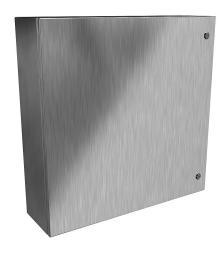
Hammond Eclipse series enclosure, NEMA 3R/4/4X/12/13,  $30 \times 30 \times 8$  in (HxWxD), wall mount, 304 stainless steel, #4 brush finish, single-door, 1/4-turn semi-flush 316 stainless steel latch.
