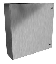
Hammond Eclipse series enclosure, NEMA 3R/4/4X/12/13, 30 x 30 x 8in (HxWxD), wall mount, 316 stainless steel, #4 brush finish, single-door, 1/4-turn semi-flush 316 stainless steel latch.
