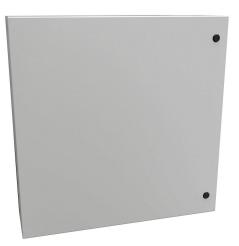
Hammond Eclipse series enclosure, NEMA 3R/4/12, 30 x 30 x 8in (HxWxD), wall mount, carbon steel, RAL 7035 light gray, powder coat finish, single-door, 1/4-turn semi-flush latch.
