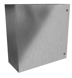
Hammond Eclipse series enclosure, NEMA 3R/4/4X/12/13,  $30 \times 30 \times 12$ in (HxWxD), wall mount, 304 stainless steel, #4 brush finish, single-door, 1/4-turn semi-flush 316 stainless steel latch.
