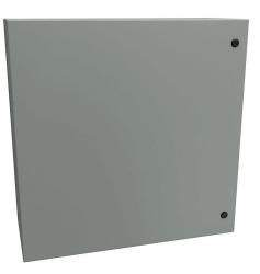
Hammond Eclipse series enclosure, NEMA 3R/4/12, 30 x 30 x 12in (HxWxD), wall mount, carbon steel, ANSI 61 gray, powder coat finish, single-door, 1/4-turn semi-flush latch.
