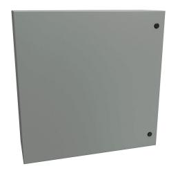
Hammond Eclipse series enclosure, NEMA 3R/4/12, 30 x 30 x 10in (HxWxD), wall mount, carbon steel, ANSI 61 gray, powder coat finish, single-door, 1/4-turn semi-flush latch.
