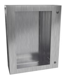
Hammond Eclipse series enclosure, NEMA 3R/4/4X/12/13,  $30 \times 24 \times 8$  in (HxWxD), wall mount, 304 stainless steel, #4 brush finish, single-door, 1/4-turn semi-flush 316 stainless steel latch, polycarbonate window.
