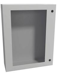
Hammond Eclipse series enclosure, NEMA 3R/4/12, 30 x 24 x 8in (HxWxD), wall mount, carbon steel, RAL 7035 light gray, powder coat finish, single-door, 1/4-turn semi-flush latch, polycarbonate window.
