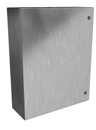
Hammond Eclipse series enclosure, NEMA 3R/4/4X/12/13, 30 x 24 x 8in (HxWxD), wall mount, 316 stainless steel, #4 brush finish, single-door, 1/4-turn semi-flush 316 stainless steel latch.
