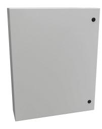
Hammond Eclipse series enclosure, NEMA 3R/4/12,  $30 \times 24 \times 6$ in (HxWxD), wall mount, carbon steel, RAL 7035 light gray, powder coat finish, single-door, 1/4-turn semi-flush latch.
