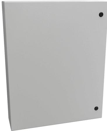
Hammond Eclipse series enclosure, NEMA 3R/4/12, 30 x 24 x 6in (HxWxD), wall mount, carbon steel, RAL 7035 light gray, powder coat finish, single-door, 1/4-turn semi-flush latch.
