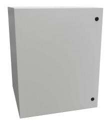
Hammond Eclipse series enclosure, NEMA 3R/4/12,  $30 \times 24 \times 24$  in (HxWxD), wall mount, carbon steel, RAL 7035 light gray, powder coat finish, single-door, 1/4-turn semi-flush latch.
