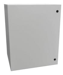
Hammond Eclipse series enclosure, NEMA 3R/4/12,  $30 \times 24 \times 20$ in (HxWxD), wall mount, carbon steel, RAL 7035 light gray, powder coat finish, single-door, 1/4-turn semi-flush latch.
