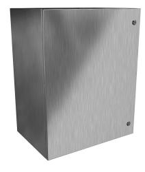
Hammond Eclipse series enclosure, NEMA 3R/4/4X/12/13,  $30 \times 24 \times 16$  in (HxWxD), wall mount, 304 stainless steel, #4 brush finish, single-door, 1/4-turn semi-flush 316 stainless steel latch.
