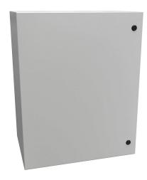
Hammond Eclipse series enclosure, NEMA 3R/4/12,  $30 \times 24 \times 16$ in (HxWxD), wall mount, carbon steel, RAL 7035 light gray, powder coat finish, single-door, 1/4-turn semi-flush latch.
