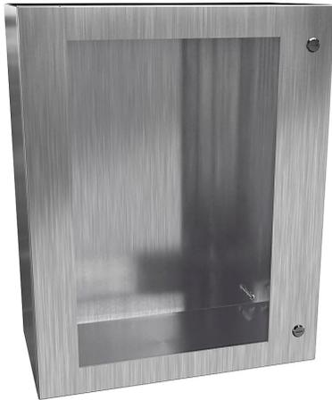
Hammond Eclipse series enclosure, NEMA 3R/4/4X/12/13, 30 x 24 x 12in (HxWxD), wall mount, 304 stainless steel, #4 brush finish, single-door, 1/4-turn semi-flush 316 stainless steel latch, polycarbonate window.
