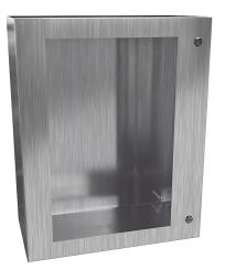
Hammond Eclipse series enclosure, NEMA 3R/4/4X/12/13,  $30 \times 24 \times 12in$  (HxWxD), wall mount, 304 stainless steel, #4 brush finish, single-door, 1/4-turn semi-flush 316 stainless steel latch, polycarbonate window.
