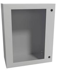
Hammond Eclipse series enclosure, NEMA 3R/4/12, 30 x 24 x 12in (HxWxD), wall mount, carbon steel, RAL 7035 light gray, powder coat finish, single-door, 1/4-turn semi-flush latch, polycarbonate window.
