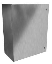
Hammond Eclipse series enclosure, NEMA 3R/4/4X/12/13,  $30 \times 24 \times 12$ in (HxWxD), wall mount, 304 stainless steel, #4 brush finish, single-door, 1/4-turn semi-flush 316 stainless steel latch.
