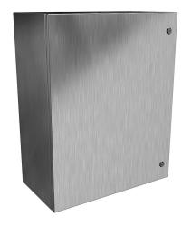
Hammond Eclipse series enclosure, NEMA 3R/4/4X/12/13, 30 x 24 x 12in (HxWxD), wall mount, 316 stainless steel, #4 brush finish, single-door, 1/4-turn semi-flush 316 stainless steel latch.
