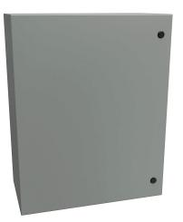
Hammond Eclipse series enclosure, NEMA 3R/4/12, 30 x 24 x 12in (HxWxD), wall mount, carbon steel, ANSI 61 gray, powder coat finish, single-door, 1/4-turn semi-flush latch.
