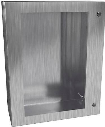
Hammond Eclipse series enclosure, NEMA 3R/4/4X/12/13, 30 x 24 x 10in (HxWxD), wall mount, 304 stainless steel, #4 brush finish, single-door, 1/4-turn semi-flush 316 stainless steel latch, polycarbonate window.
