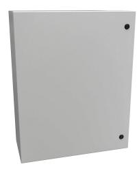
Hammond Eclipse series enclosure, NEMA 3R/4/12,  $30 \times 24 \times 10$ in (HxWxD), wall mount, carbon steel, RAL 7035 light gray, powder coat finish, single-door, 1/4-turn semi-flush latch.
