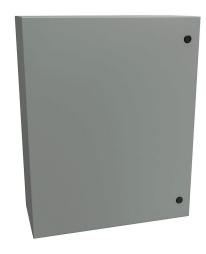
Hammond Eclipse series enclosure, NEMA 3R/4/12, 30 x 24 x 10in (HxWxD), wall mount, carbon steel, ANSI 61 gray, powder coat finish, single-door, 1/4-turn semi-flush latch.
