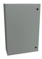
Hammond Eclipse series enclosure, NEMA 3R/4/12,  $30 \times 20 \times 8in$  (HxWxD), wall mount, carbon steel, ANSI 61 gray, powder coat finish, single-door, 1/4-turn semi-flush latch.
