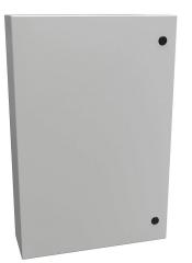
Hammond Eclipse series enclosure, NEMA 3R/4/12, 30 x 20 x 6in (HxWxD), wall mount, carbon steel, RAL 7035 light gray, powder coat finish, single-door, 1/4-turn semi-flush latch.
