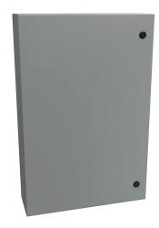
Hammond Eclipse series enclosure, NEMA 3R/4/12,  $30 \times 20 \times 6$ in (HxWxD), wall mount, carbon steel, ANSI 61 gray, powder coat finish, single-door, 1/4-turn semi-flush latch.
