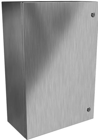
Hammond Eclipse series enclosure, NEMA 3R/4/4X/12/13, 30 x 20 x 10in (HxWxD), wall mount, 304 stainless steel, #4 brush finish, single-door, 1/4-turn semi-flush 316 stainless steel latch.
