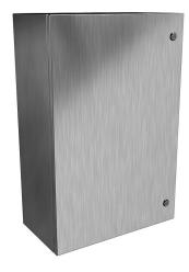
Hammond Eclipse series enclosure, NEMA 3R/4/4X/12/13,  $30 \times 20 \times 10$  in (HxWxD), wall mount, 316 stainless steel, #4 brush finish, single-door, 1/4-turn semi-flush 316 stainless steel latch.
