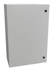
Hammond Eclipse series enclosure, NEMA 3R/4/12, 30 x 20 x 10in (HxWxD), wall mount, carbon steel, RAL 7035 light gray, powder coat finish, single-door, 1/4-turn semi-flush latch.
