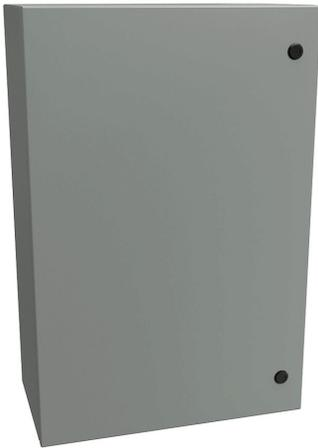
Hammond Eclipse series enclosure, NEMA 3R/4/12, 30 x 20 x 10in (HxWxD), wall mount, carbon steel, ANSI 61 gray, powder coat finish, single-door, 1/4-turn semi-flush latch.
