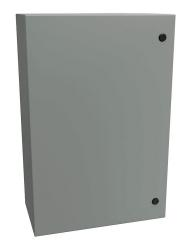
Hammond Eclipse series enclosure, NEMA 3R/4/12, 30 x 20 x 10in (HxWxD), wall mount, carbon steel, ANSI 61 gray, powder coat finish, single-door, 1/4-turn semi-flush latch.
