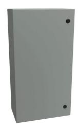
Hammond Eclipse series enclosure, NEMA 3R/4/12,  $30 \times 16 \times 8$ in (HxWxD), wall mount, carbon steel, ANSI 61 gray, powder coat finish, single-door, 1/4-turn semi-flush latch.
