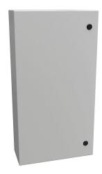
Hammond Eclipse series enclosure, NEMA 3R/4/12,  $30 \times 16 \times 6$ in (HxWxD), wall mount, carbon steel, RAL 7035 light gray, powder coat finish, single-door, 1/4-turn semi-flush latch.
