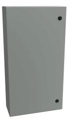
Hammond Eclipse series enclosure, NEMA 3R/4/12, 30 x 16 x 6in (HxWxD), wall mount, carbon steel, ANSI 61 gray, powder coat finish, single-door, 1/4-turn semi-flush latch.
