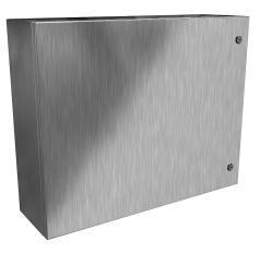
Hammond Eclipse series enclosure, NEMA 3R/4/4X/12/13, 24 x 30 x 8in (HxWxD), wall mount, 304 stainless steel, #4 brush finish, single-door, 1/4-turn semi-flush 316 stainless steel latch.
