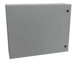
Hammond Eclipse series enclosure, NEMA 3R/4/12,  $24 \times 30 \times 8in$  (HxWxD), wall mount, carbon steel, ANSI 61 gray, powder coat finish, single-door, 1/4-turn semi-flush latch.
