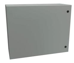
Hammond Eclipse series enclosure, NEMA 3R/4/12,  $24 \times 30 \times 12$ in (HxWxD), wall mount, carbon steel, ANSI 61 gray, powder coat finish, single-door, 1/4-turn semi-flush latch.
